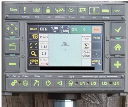
The screen and controls of a Javad Triumph-LS survey grade GPS device
